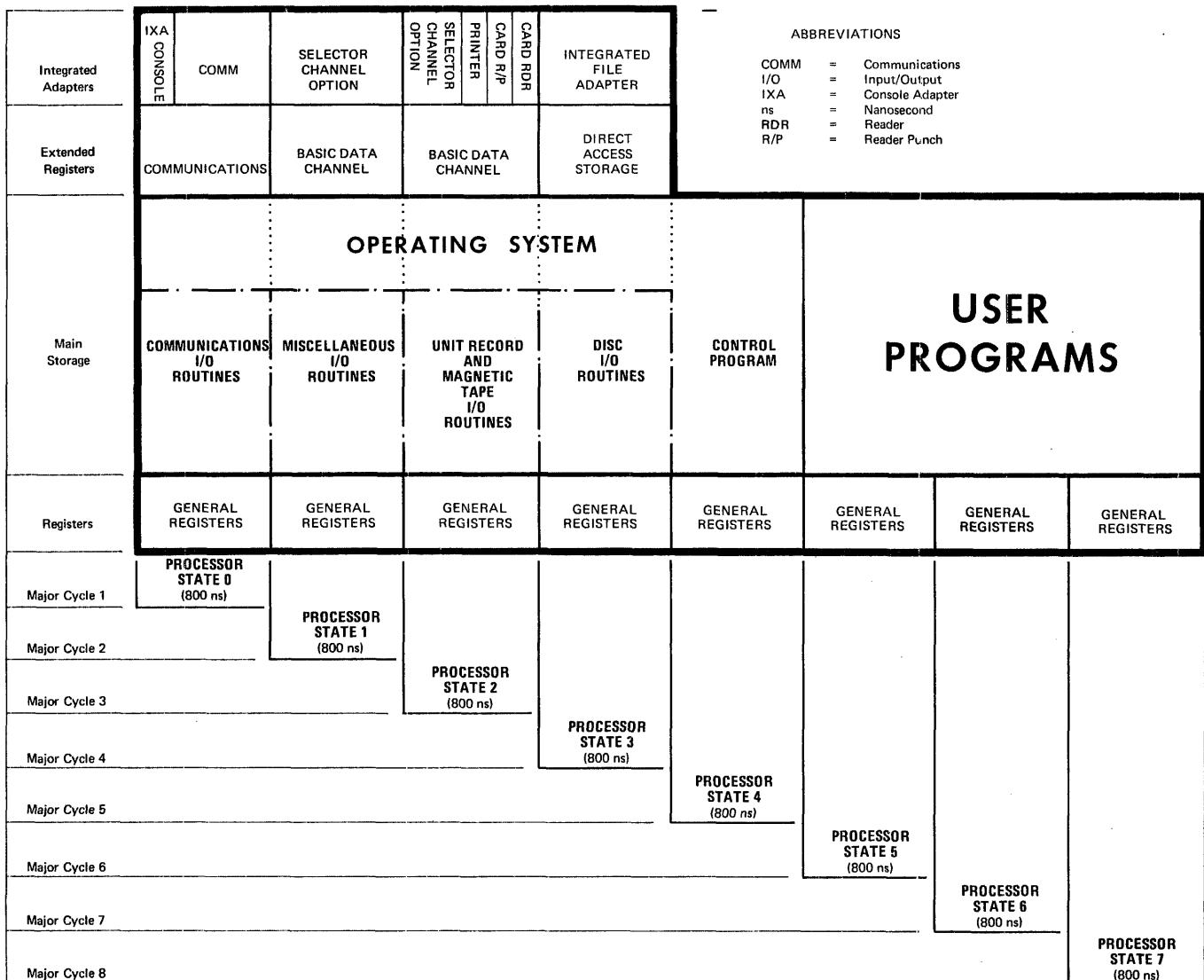
**Figure 2-1. System Architecture**
